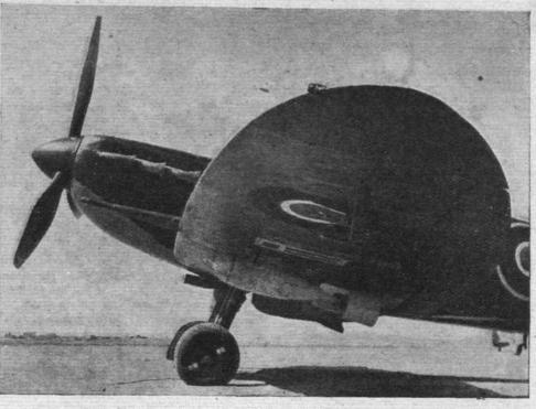
CANNON AND BOMB: A mark V Spitfire with 250 lb. bombs fitted under the wing. This famous fighter now provides height-cover and zero-ft. strafing.
